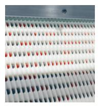
The **CountSafe™ - Slat Counter** can inspect: tablets, capsules, gel caps, dual colored capsules and dual colored tablets. This cost-effective, ergonomically designed **CountSafe™ - Slat Counter** detects wrong color, missing, broken, chipped or over/ undersized tablets, foreign object/material and overall product integrity.
